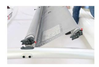
6) ... put it on the side of the middle beam, fix it with the knee and fasten it with the Velcro.
