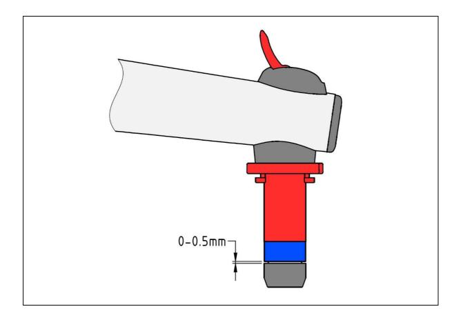
Info: Regularly grease the friction surface of the clamping levers with lubricating grease (e.g. Vaseline) to keep them running smoothly.
