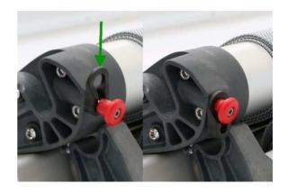
12) Pull front crossbar out of one hull first and lay the hull aside.
