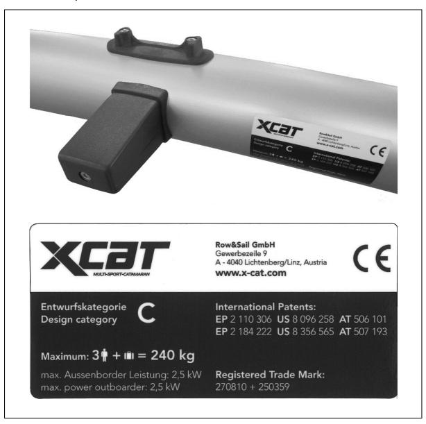
The identification number is located on the rear side of the hull after the flange.
