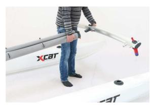
11) Pull off the center section from the front crossbeam.
