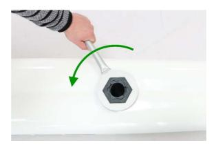
2) Pull flange out of hull and drain hull with opening facing down.
