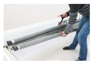
11) First unroll the side beam rolled up on the side, ...
