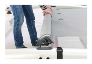
5) On the other side, unlock the rear locking bolt and unhook the side beam, then roll up downward, ...
